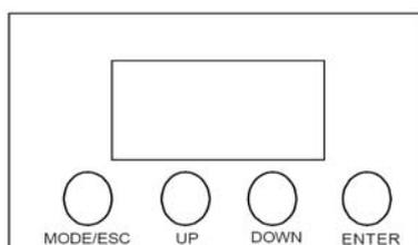
The main menu is accessed by pressing the Mode/Esc-button, Browse through the submenu by pressing Up or Down. Press the Enter-button in order to select the desired menu. You can change the selection by pressing Up or Down, Confirm every selection by pressing the Enter-button. You can leave every mode by pressing the Mode/Esc-button. The functions provided are described in the following setting.
