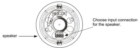
3. After simultaneously pressing the fixed springs on both sides of the ceiling speaker to the end push it into the round hole of the ceiling and then the speaker is fixed.
