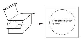
Ceiling hole drilling size
